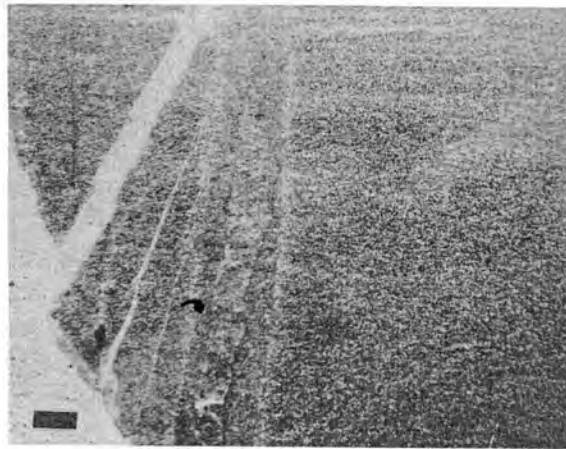
Micrograph of pelletal lime grainstone, (Tc) current ripple laminations (lower) (Tc) laminations (upper). Vertical burrow is about 2 mm in diameter. Unnamed Kee (1976), Toquima Range. Bar is 1 mm.
