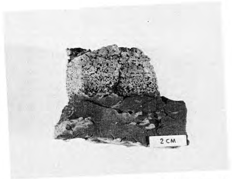
Figure 16. Incompletely silicified, case hardened grapestone overlying carbonate mud/wackestone. Unit 21 of this study, Paris Peak Member, Fish Haven Dolomite, Lakeside Mountains.
